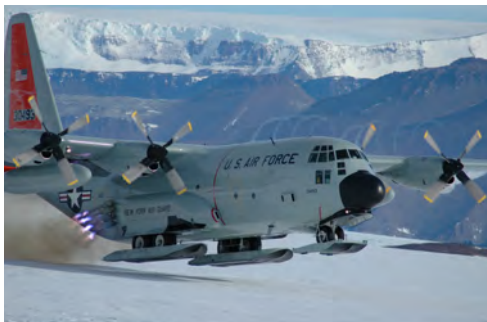
LC130 Hercules transport plane used as part of the Ice Pod project in both poles. Altitude 30,000 ft. - Payload 30,000 lbs.
